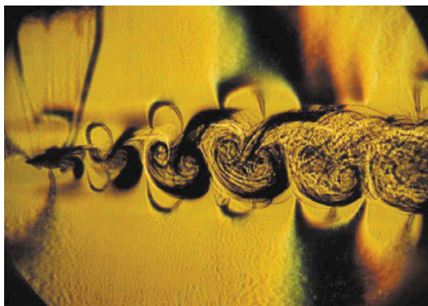
Fig. 3. Strongly stratified fluid, T_b = 7.5 s. Strip is sloped under the angle \alpha = 16^\circ to horizontal and is towed with velocity U = 4.21 cm/s. Strong anisotropy of turbulent vortex array is observed. Light and dark strips across the image visualize attached internal waves. Boundaries between light and dark areas near and past the strip are crests and troughs of attached internal waves.
